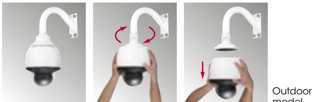
Remove Top Sunshade, Rotate Main Unit and pull (Need to remove locking screws)
